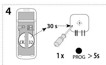
Remove the battery from the detector again. After 30 seconds, press the programming button for more than 5 seconds to bring the compatible component into timer mode. LED 2x blinks at second intervals. When the button is released, delayed return time is retrieved.
