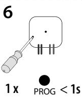
Press of programming button on compatible actuator shorter then 1 second will finish programming mode, LED switches off.
