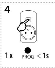
End learning mode by a short press of the programming button on the RFRP-20. By doing so, the programmed detector address is stored in the memory. The red LED will flash for 1 second, then the green LED will remain illuminated.
