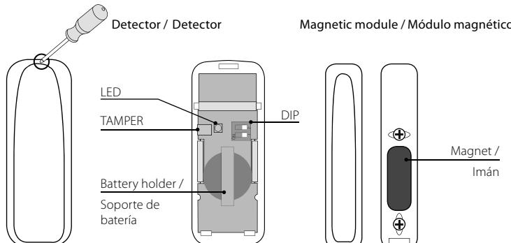
Before starting to program, open the detector cover using a screwdriver. Indicators and adjustment components are located inside the box.
