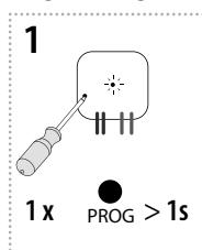
Press of programming button on compatible actuator for 1 second will activate actuator into programming mode. LED is flashing in 1s interval.
