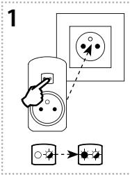
When inserting the RFRP-20 into an electrical socket (upon power-up), the programming button must be pressed. The green LED flashes. Then when the red LED illuminates, release the button.
