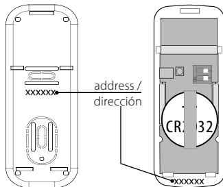
For programming and communicating the detector with the system components, the address shown on the underside of the detector or at the bottom of the open device is used.
