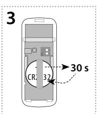
Remove the battery from the detector and reinser it after 30 seconds. The red LED on the detector will blink. The LED on a compatible component will flash at a faster interval.
