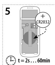
After setting the desired time (within 2s ... 60min), the timer mode ends by inserting the battery into the detector. The red LED on the detector will blink. This saves the time interval stored in the memory of the component, the LED on the compatible component blinks.
