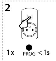
By one short press of the programming button on the RFRP-20, you move to the position for input into the additional learning mode. The red LED flashes - after 5s the RFRP-20 enters the additional learning mode. The LED stops flashing.
