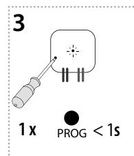
Press of programming button on compatible actuator shorter than 1 second will finish programming mode, LED switches off.
