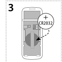
Insert the battery into the battery holder in the detector (Beware of the polarity, the red LED on the detector will blink). A flashing green LED on the RFRP-20 indicates that the RFWD-100 has been recorded in the RFRP-20 memory.
