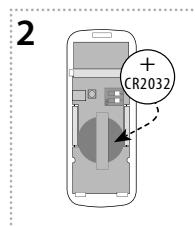
Slide the battery into the battery holder in the detector. Beware of the polarity. The red LED on the detector will blink. The LED on a compatible component will blink at a faster interval - thereby assigning the detector to the component.
