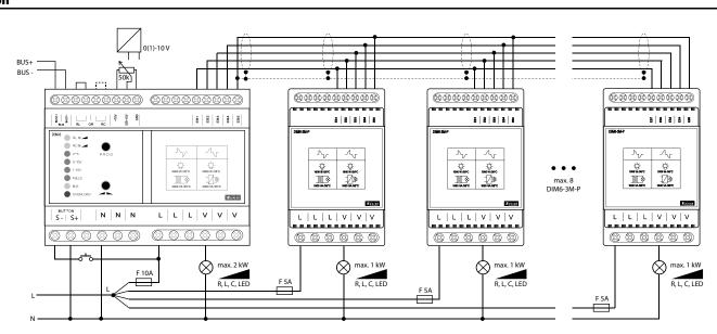
A quick fuse corresponding to the power of each module must be included in the L supply for each module.
